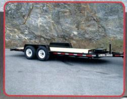
The easiest way to load and unload equipment is now available in the Bri-Mar Hydraulic Tilt Series. No need for ramps, just drive onto the low angle deck and the hydraulic cylinder does the rest. Any easier and it would load the equipment for you.
